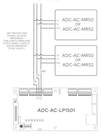
For ease of install, daisy chain expansion modules together. Wire each expansion module to the next module instead of wiring directly back to the controller.
